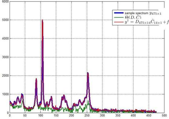
Fig. 2. Spectra plots for the sample spectrum  $y_{475 \times 1}$  (blue), library contribution  $\Theta(X, C)$  (green) and reconstructed spectrum  $y^\dagger = f + \Theta(X, C)$  (red). The sample is a mixture of potentially dangerous chemicals that is of interest to DSTL.
